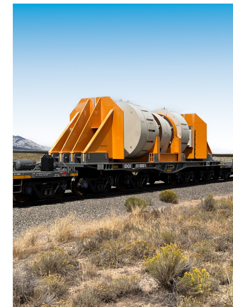
Atlas Railcars will be used to transport used nuclear fuel across the country.
