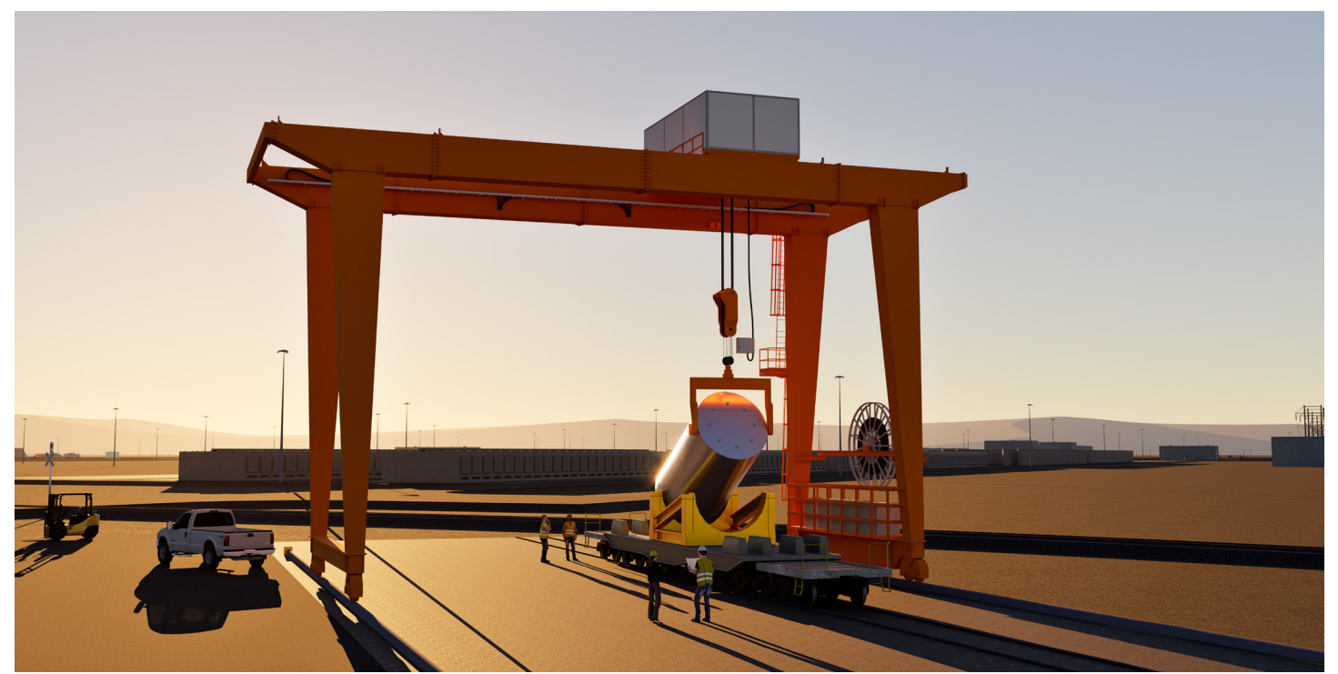
Concept of unloading a transportation cask at a Federal staging facility for used nuclear fuel.
